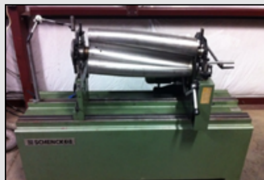
All Scrolls Are Precision Balanced
