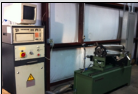
All Rebuilt Roots Blowers are Bench Tested
