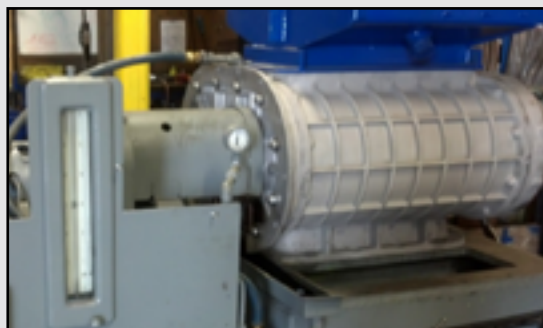
All Rebuilt Roots Blowers are Bench Tested
